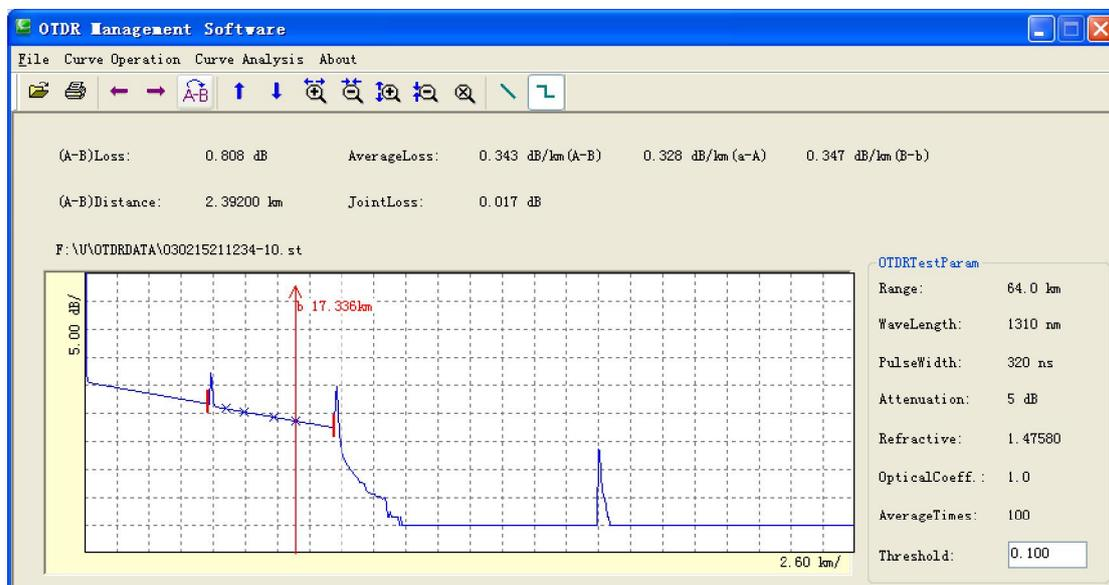
The real time loss and wave form display area when it is testing the joint loss
