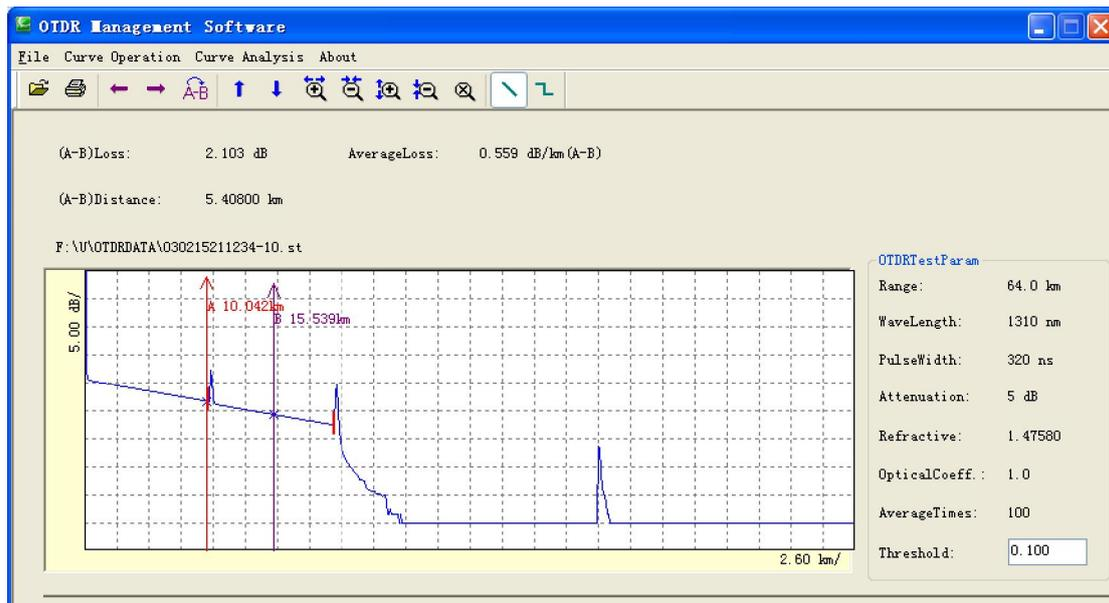
The real time loss and wave form display area when it is testing the average loss
