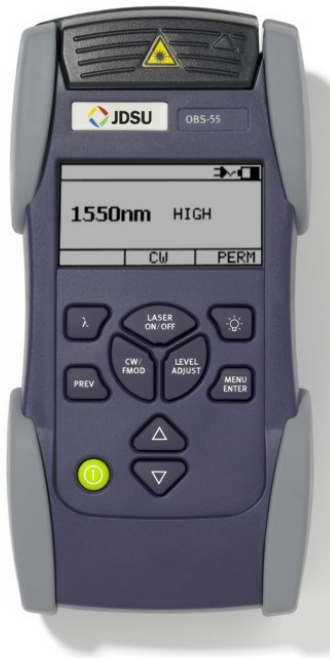
OBS-55: For PMD and Attenuation Profile measurement
